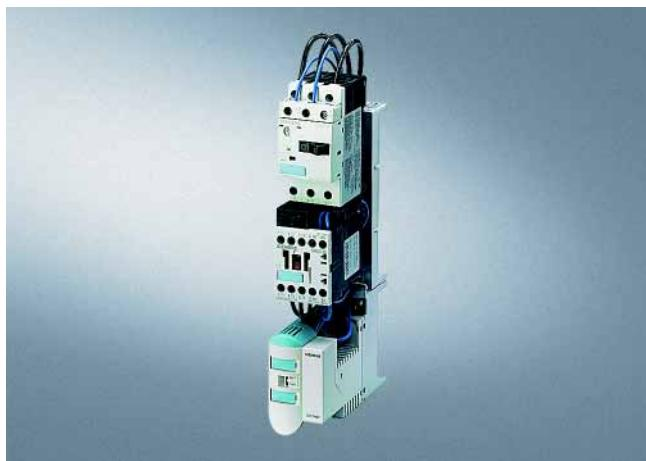
The 3RA5 fuseless load feeders with AS-Interface offer the possibility of linking motor starters swiftly and at low cost to higher-level automation systems. The integrated 3RV1 motor starter protector for motor protection protects the motor against overloads and provides short-circuit protection for the cables. The 3RT1 contactor is used for operational switching. The switching state is triggered and signaled using the 3RK1 4 load feeder module on the AS-Interface.
